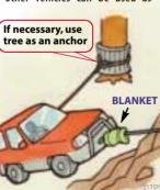
anchors, but natural objects such as trees, stumps and rocks are best. Select the anchor carefully and ensure it can withstand the load.
