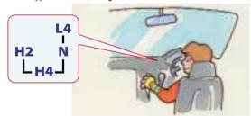
As a general rule, shifting into 4WD is to be done while the car is parked. Yet, there are types of 4WD that allow the shifting to be done while the vehicle is in motion. Confirm the appropriate procedure (by consulting the operation manual) so as not to damage the vehicle and to avoid accidents. When the shift is made, usually an indicator lamp lights up to confirm the shift. However, the lamp can fail and driving the car is a better way of confirming that the shift into 4WD has taken place.
