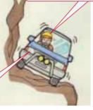
Steer to the valley side to adjust the direction of the vehicle.
